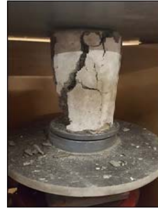
Figure 6. Concrete breaking test in ASI frame
