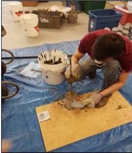
Figure 4. Molding of cylinders for strength testing
