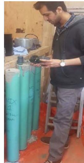
Figure 7. PIT testing on miniature pile models
