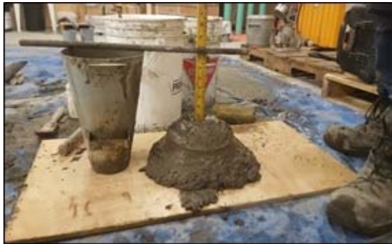
Figure 5. Slump Test conducted on mix design 1
